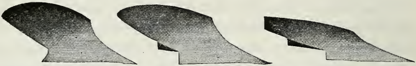
Fig. 108. The three principal types of plows, showing in order the stubble, the general purpose, and the prairie breaker plows.
