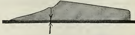
Fig. 110. Illustrating method of using a straight-edge to determine whether a plow has the proper "suction."
