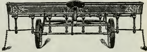
Fig. 136. A broadcast seeder with a narrow-track truck.
