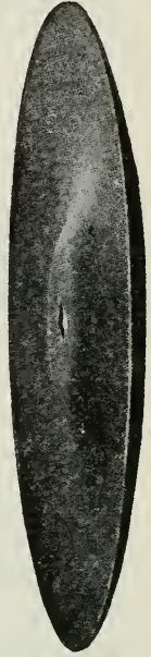
Fig. 126. A plow-cut disk used on disk harrows. Note the raised center.
